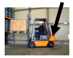
• Any mass being lifted at the front will create an anticlockwise torque about a pivot point such as the front wheel of the fork lift.
